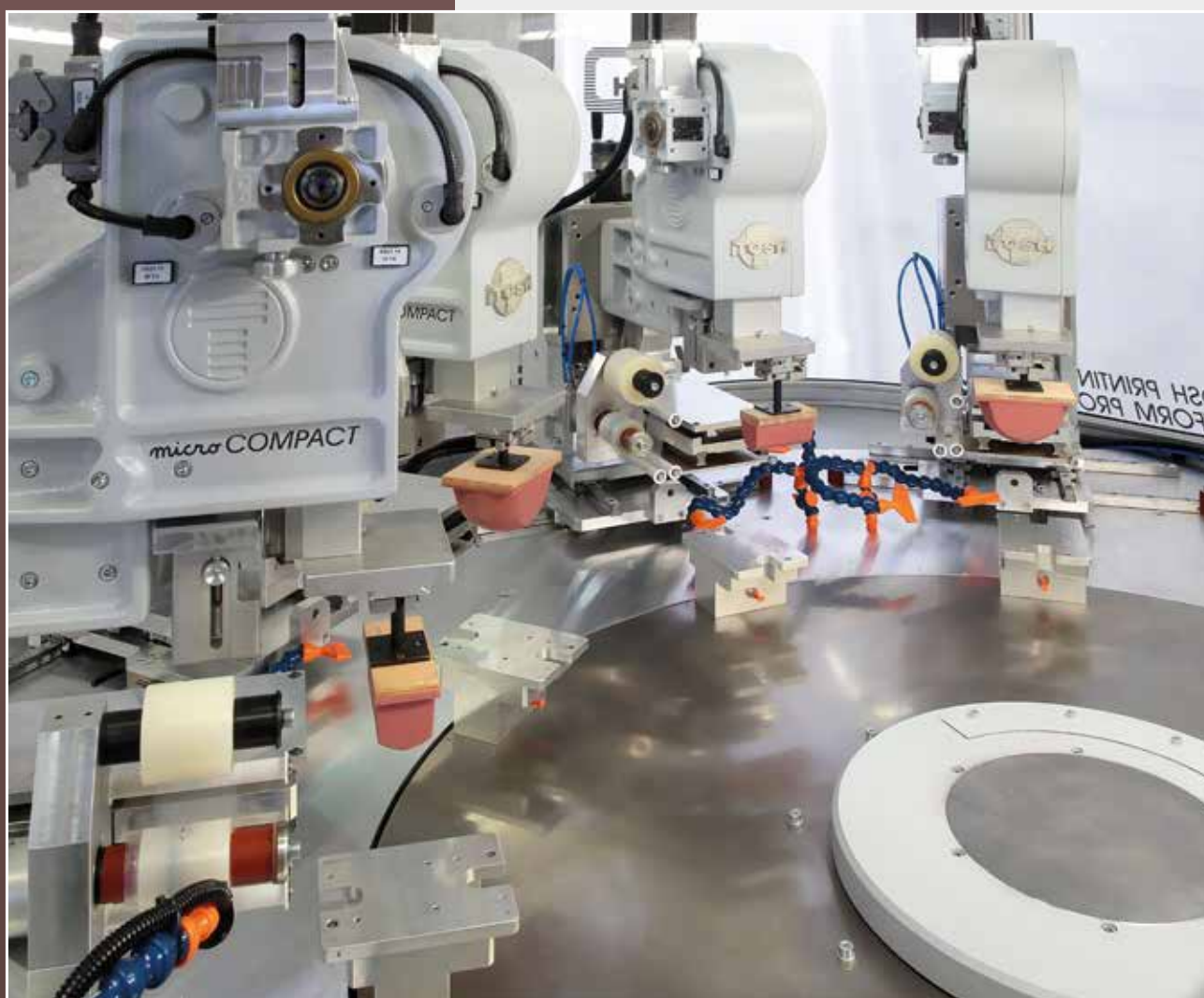
N. 4 Logica Micro Compact 1 colour with automatic pad cleaning device on numerically controlled rotary table.
