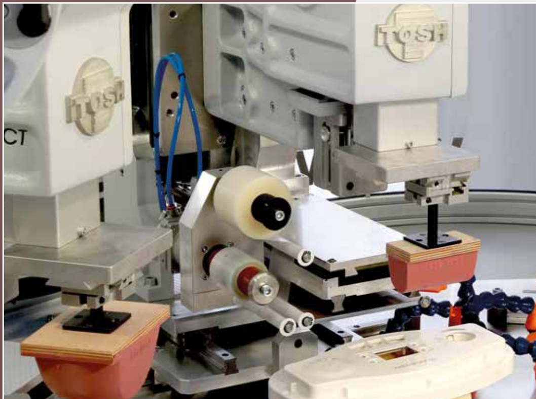
N. 2 Logica Micro Compact 1 colour with automatic pad cleaning device on numerically controlled rotary table
