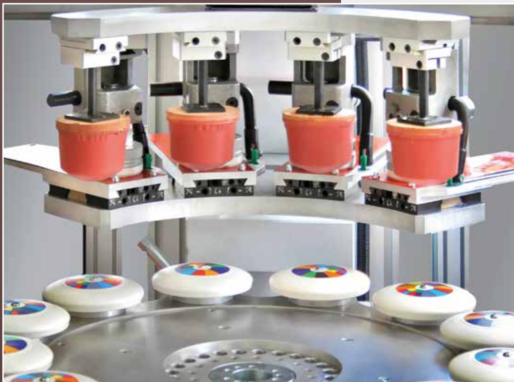
Four colours radial plate configuration with numerically controlled rotary table
